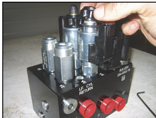
FIGURE 20. Coil Reinstalled on the AutoBoom Valve
