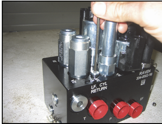
FIGURE 29. Port Plug Reinstalled on the AutoBoom Valve
