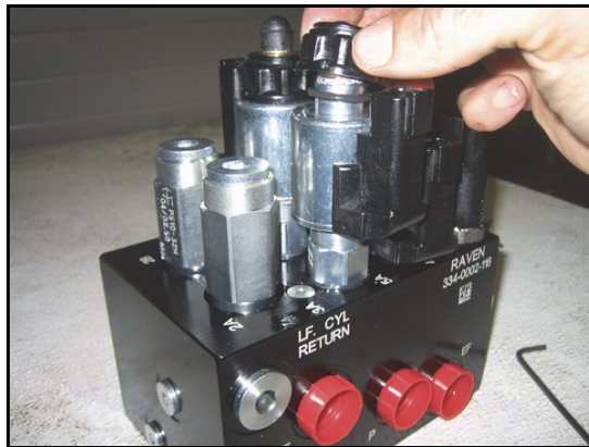
FIGURE 8. Coil Reinstalled on the AutoBoom Valve
