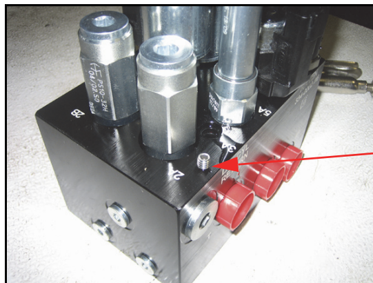
FIGURE 18. Orifice Fitting Removed from the AutoBoom Valve
