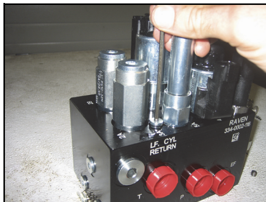
FIGURE 6. Port Plug Reinstalled on the AutoBoom Valve
