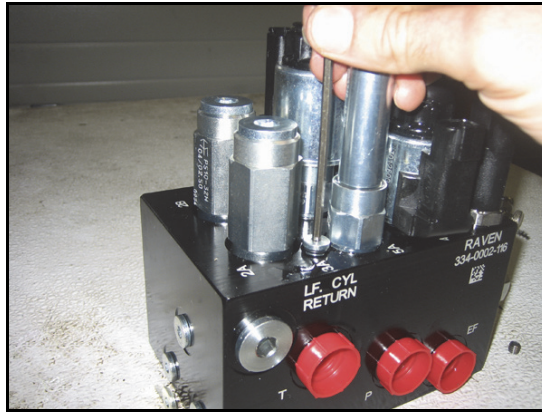
FIGURE 7. Port Plug Reinstalled on the AutoBoom Valve
