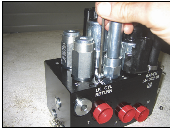
FIGURE 19. Port Plug Reinstalled on the AutoBoom Valve
