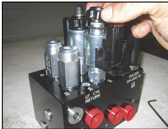
FIGURE 30. Coil Reinstalled on the AutoBoom Valve
