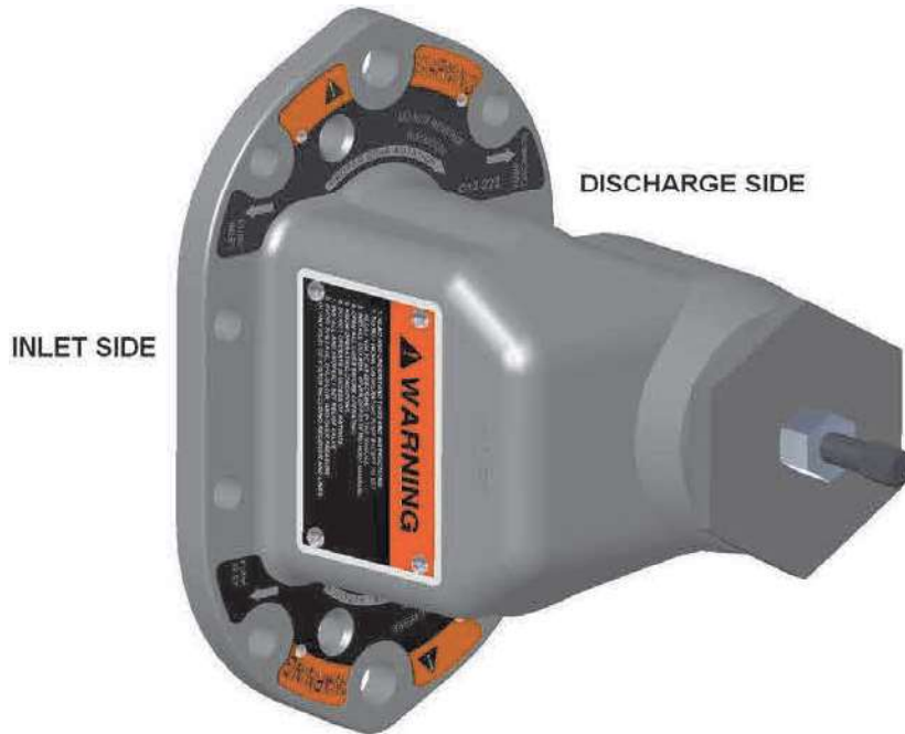
FACEPLATE ASSEMBLY FOR RV STYLE SINGLE DIRECTION RELIEF VALVE FIGURE 5.3
