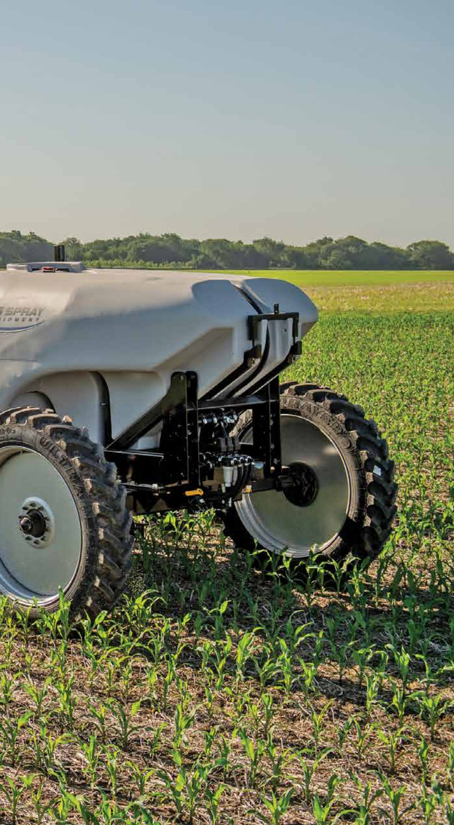
Double Cylinder Allows The Gullwing & Main Lift To Be Controlled With One Hydraulic Remote
