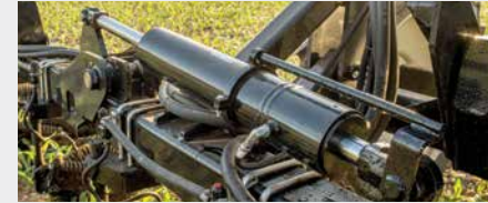
Auto Gull Wing function allows the wings of the bar to automatically tilt up when main bar is raised for greater turning clearance.
