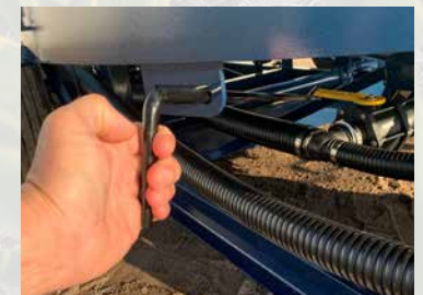
Valve handle extension standard on all Single, Double and Triple Cone Trailers.
